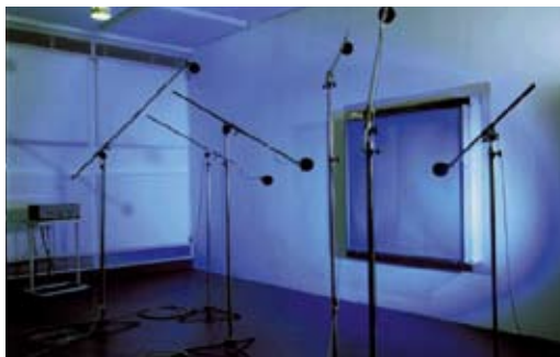
Noise measurements to DIN 45 635-38 „Noise Measurement of Machines: Fans“
